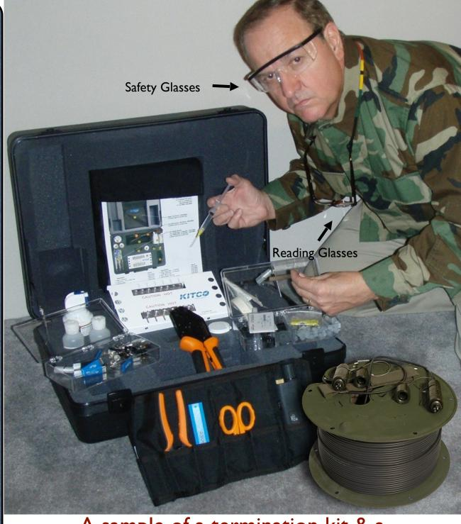
A sample of a termination kit & a reel of TFOCA II® fiber!
