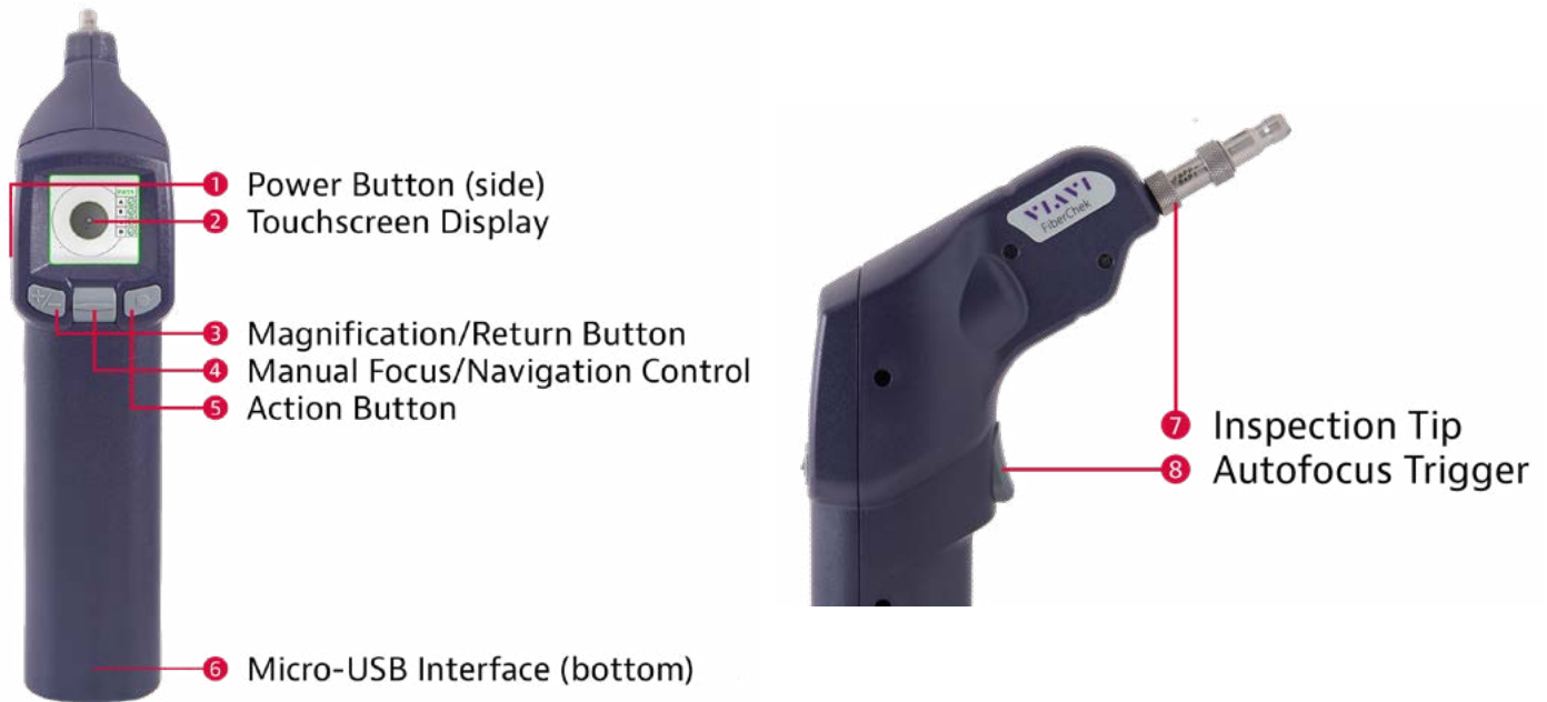
Figure 3-1 – FiberChek Probe Controls and Display
